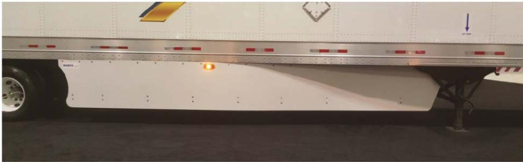
30. Defendants’ accused trailer skirts also include, for example as set forth in Claim 1 of the ’471 patent, a front portion having a front height and the rear portion having a rear height, the front height being shorter than the rear height, as shown below.
