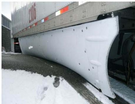
Further, the resilient struts are characterized in that they can sustain substantial elastic deformation when the skirt panel is impacted by a foreign object and to return substantially to the original position when the skirt panel is no longer being impacted by the foreign object. For
