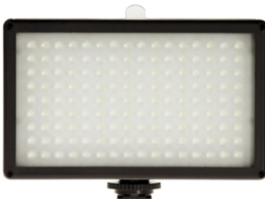
19. iLED 144 products include 144 LEDs arranged in alternating columns of warm and cool white LEDs. The warm white LEDs have a color temperature of 3200 K and the cool white LEDs have a color temperature of 5600 K.
