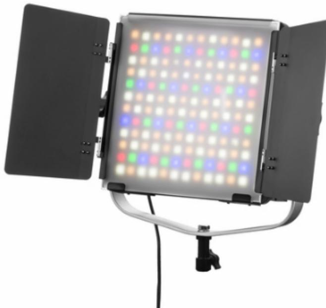
58. Multi-K XL products include 144 LEDs, comprised of red, green, blue, warm white, and cool white LEDs. The warm white LEDs have a color temperature of 3200 K and the cool white LEDs have a color temperature of 5600 K.
