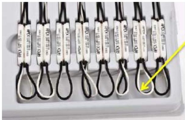
15. As further recited by claim 1 of the '140 patent, each module of the AgiLight SignRayz products includes "a first support comprising a dielectric layer and circuitry" as illustrated in the photograph below of an AgiLight SignRayz module with the over-molding removed to which a red arrow has been added to identify the first support:
