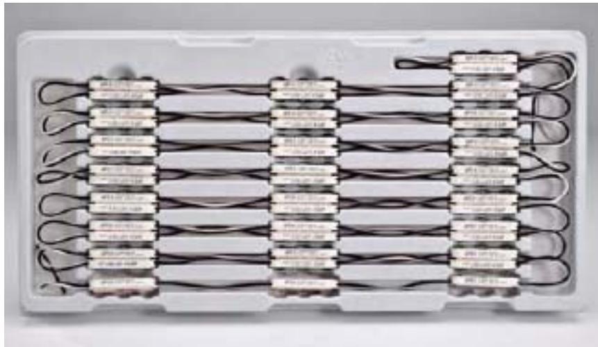
65. As further recited by claim 16 of the '896 patent, the modules of the AgiLight SignRayz Series G2 “LED modules includ[e] a support having circuitry on a first surface.” This is shown by the fact that each LED module has a support comprising a printed circuit board having circuitry on a surface of the PCB as illustrated in the photograph below:
